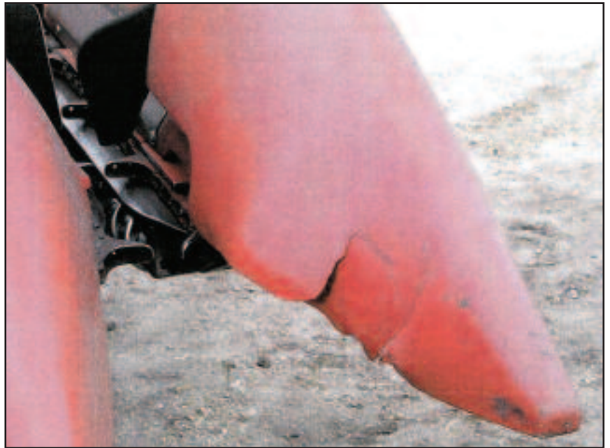
Damage to equipment after sinking in soft soil in trench.
